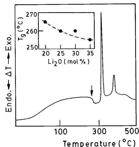
FIG. 3. Differential thermal analysis curve of  $30\text{Li}_2\text{O}-70\text{Bi}_2\text{O}_3$  glass composition. Inset shows the variation of  $T_g$  with the  $\text{Li}_2\text{O}$  content in the glass composition.
