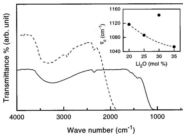
FIG. 6. FTIR spectra of 30Li<sub>2</sub>O-70Bi<sub>2</sub>O<sub>3</sub> (solid curve) and PbO-Bi<sub>2</sub>O<sub>3</sub> (dashed curve) glasses. Inset shows the variation of  $\bar{\nu}_c$  with the Li<sub>2</sub>O content in the lithium bismuthate glasses.
