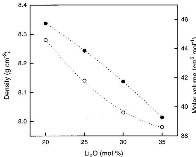
FIG. 4. Variation of density (○) and molar volume (●) with the Li<sub>2</sub>O content in the glass composition.
