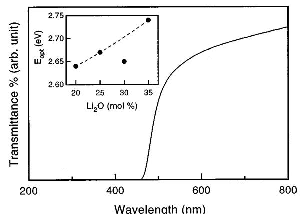
FIG. 5. Optical spectrum of 30Li<sub>2</sub>O-70Bi<sub>2</sub>O<sub>3</sub> glass composition in the UV-VIS region. Inset shows the variation of  $E_{opt}$  with the Li<sub>2</sub>O content in the glass composition.
