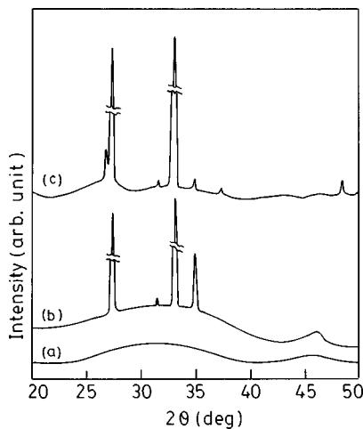
FIG. 1. X-ray-diffraction patterns of different samples: (a)  $30\text{Li}_2\text{O}-70\text{Bi}_2\text{O}_3$  sample as prepared, (b)  $30\text{Li}_2\text{O}-70\text{Bi}_2\text{O}_3$  sample heat treated at  $340^\circ\text{C}$ , and (c)  $30\text{Li}_2\text{O}-70\text{Bi}_2\text{O}_3$  sample heat treated at  $400^\circ\text{C}$ .
