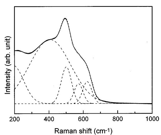
FIG. 7. Raman spectrum of 30Li<sub>2</sub>O-70Bi<sub>2</sub>O<sub>3</sub> glass composition. Deconvoluted peaks are indicated by dashed curves.
