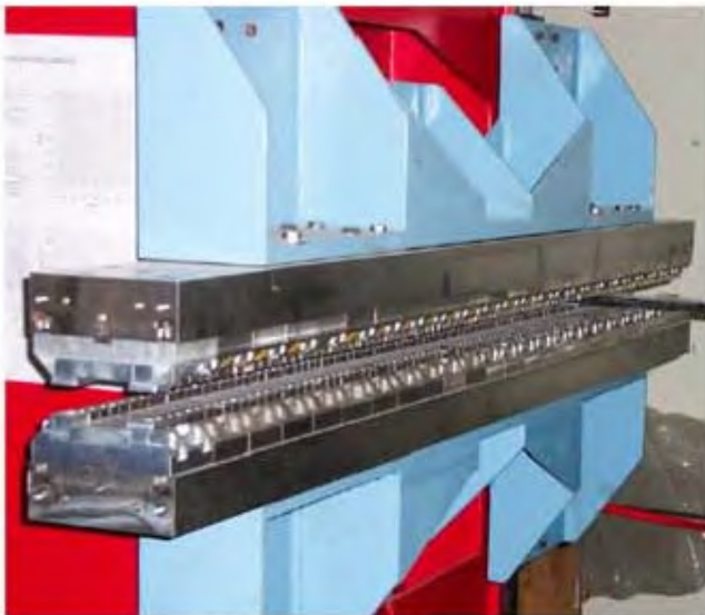
Figure 2. Photograph of a typical pure permanent magnet undulator. This one was developed at the Beam Physics and FEL Laboratory, for the CUTE-FEL. Portions in blue and red are support structure for the undulator. The magnets themselves are mounted in the steel ‘jaw’ at the centre in two arrays. The top surface of the magnets is clearly visible.
