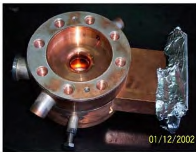
Figure 5. Photograph of a prototype photocathode rf gun structure developed at the Beam Physics and FEL Laboratory, CAT for short-wavelength FEL applications. The final gun will produce 100 A, 8 ps electron bunches and can be upgraded to higher currents and shorter pulse-lengths.
