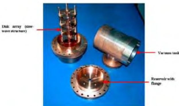
Figure 7. Components of a Plane Wave Transformer (PWT) linac structure developed at the Beam Physics FEL Laboratory. The disk array, which is responsible for producing the accelerating field, fits into the vacuum tank that has ports for RF feed and vacuum pump. The electron beam to be accelerated passes through the holes at the centre of the disks. The total length of the linac is just 21 cm, and it has successfully accelerated electrons up to 3.5 MeV.
