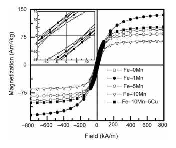
Figure 9. Magnetization vs applied magnetic field curve for as-prepared powders obtained after milling for 120 h.
