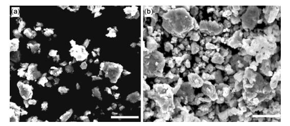
**Figure 7.** SEM micrographs of as-prepared powders after milling for 100 h: (a) Fe–0Mn and (b) Fe–1Mn. Bar = 5  $\mu$ m.
