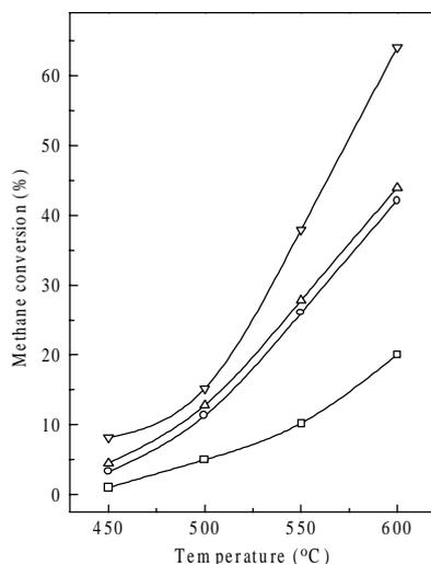
**Figure 5.** Effect of temperature on the conversion of methane in its complete combustion over  $\text{LaCoO}_3$  – treated with water at  $125^\circ\text{C}$  (○),  $175^\circ\text{C}$  (△),  $225^\circ\text{C}$  (▽) and without water treatment (□).
