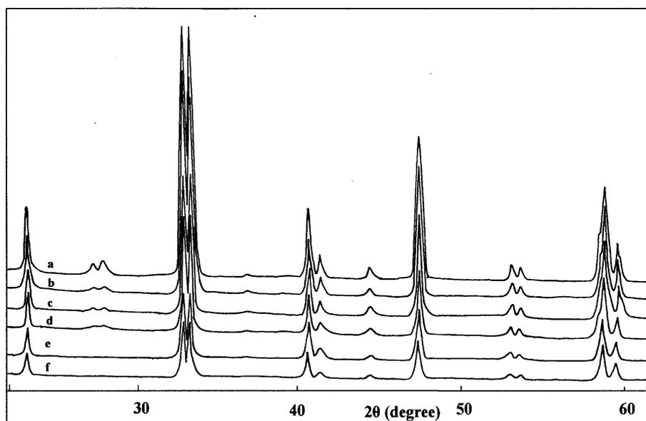
**Figure 3.** XRD spectra of LaCoO<sub>3</sub> [without treatment (a), treated with water at 125°C (b), 175°C (c), 275°C (d), with steam at 350°C (e) and 800°C (f)].
