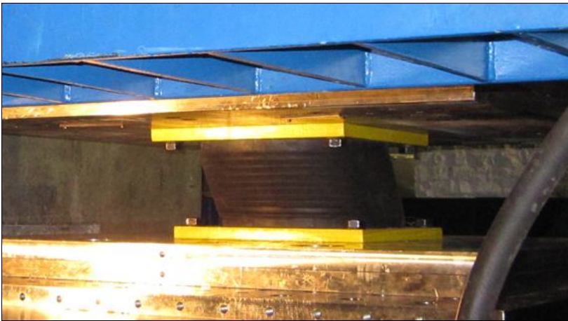
Figure 8. LRB during horizontal cyclic characteristic test
