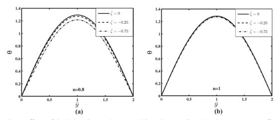
Fig. 2. Effects of the induced streaming potential on the non-dimensional temperature profiles for (a) n=0.8 (b) n=1.
