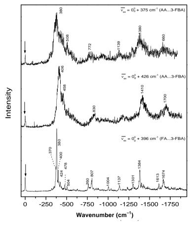
FIG. 7. Comparison of the dispersed fluorescence spectra for excitations with similar excess vibronic energy of the (a, b)  $AA\cdots 3$ -FBA mixed dimer with that of (c)  $FA\cdots 3$ -FBA dimer.
