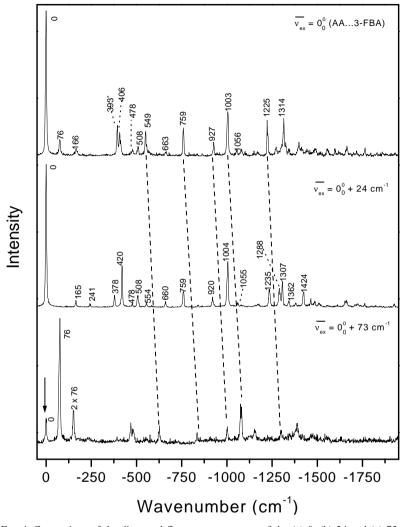
FIG. 4. Comparison of the dispersed fluorescence spectra of the (a) 0, (b) 24 and (c)  $73 \text{ cm}^{-1}$  bands of the mixed dimers.
