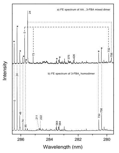
FIG. 2. Comparison of the fluorescence excitation spectra for  $S_1 \leftarrow S_0$  electronic excitations of the (a) mixed dimer AA···3-FBA and (b) homodimer (3-FBA)<sub>2</sub>. The homodimer bands in (a) are labeled by asterisks. The band-labeled 24 has been assigned as  $0_0^0$  transition of a second conformational species of the dimer.
