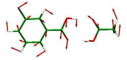
FIG. 3. The DFT-predicted mode pattern of the rocking motion of the 3-FBA moiety at the hydrogen-bonded interface. The conformer-I undergoes geometry distortion along this vibrational coordinate on  $S_1 \leftarrow S_0$  electronic excitation.
