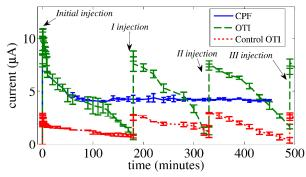
45 Fig. 5 Demonstration of the two operating modes of the device under consideration. OTI stands for one time injection (with intermittent refill injections highlighted by the peaks occurring in Fig. 5) and CPF stands for Capillary flow mode. Both these modes were tried using *P*.
