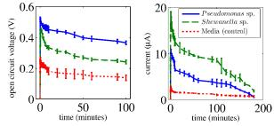
Fig. 4 (a) Temporal variation of the open circuit voltage and (b) current for the paper MFC using both *P. aeruginosa.*, *S. putrefaciens.* and control in an OTI mode.
